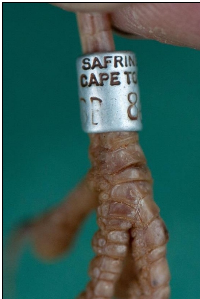
Fig. 4. At just over 2 years old, this aluminium ring already showed wear.
